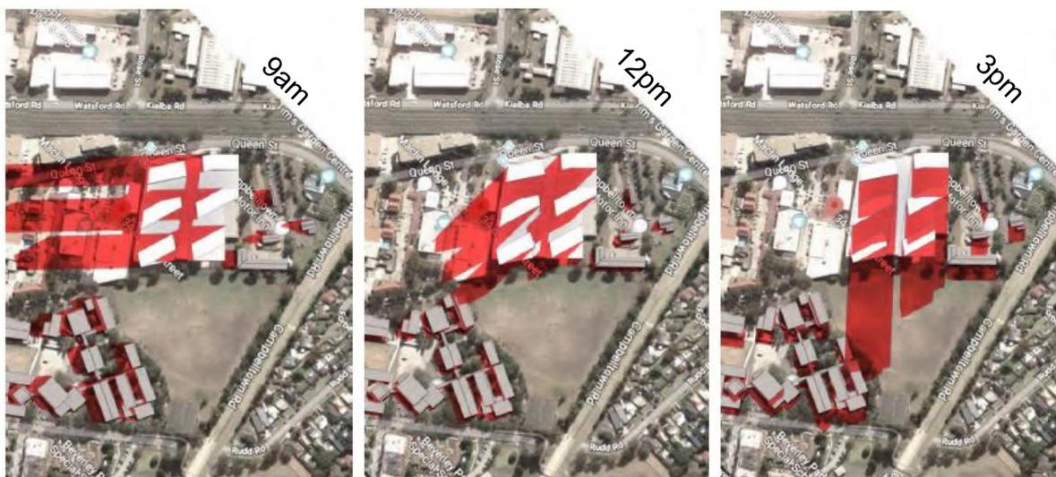
Figure 12: Shadow diagram during winter solstice.
